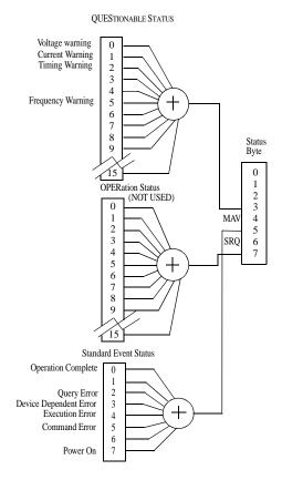
The instrument has a status reporting system conforming to IEEE 488.2 and SCPI. The figure above shows the status groups available in the instrument.
