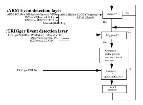
You program the comprehensive triggering capabilities of the instrument using the SCPI :ARM and :TRIGger subsystems. Using these two command subsystems you can program the operating modes of the instrument which are set up using the MODE/TRG screen on the frontpanel.
